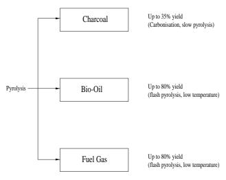
Fig. 3. Energy products from pyrolysis.
