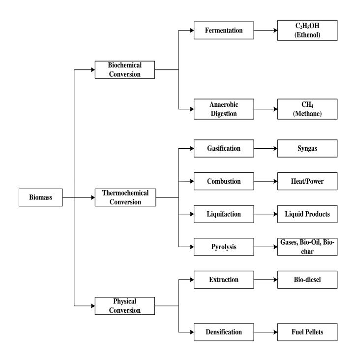
Figure-1: Conversion technologies for biomass into energy.
