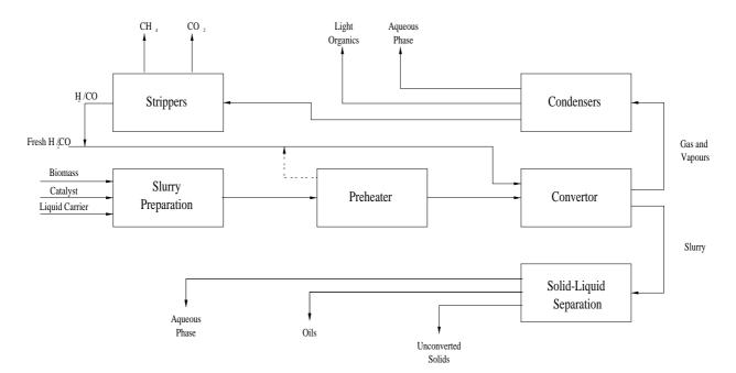
Fig. 5. Flow sheet for liquefaction.
