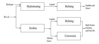
Fig. 4. Treatment and upgrading options for bio-oil.
