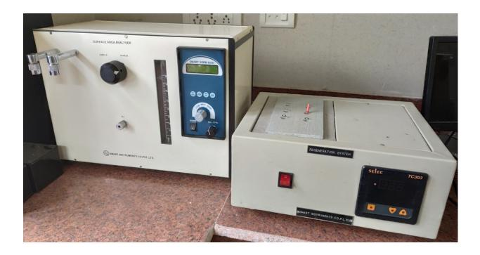
Surface area analyzer is a very sensitive technique to find out the surface area, size, shape and volume of the pores. It is also useful to calculate the catalytic activity of the solid catalyst. Surface area analyzers help researchers obtain the area or pore size of surfaces on samples as diverse as pharmaceuticals and activated carbon by measuring their gas sorption capabilities. The greater an object's surface area, the more capable it is of gas sorption.
