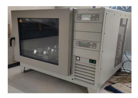
An incubator shaker (or thermal shaker) can be considered a mix of an incubator and a shaker. It has an ability to shake while maintaining optimal conditions for incubating microbes or DNA replications.
