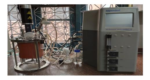
Bioreactor is a device or system that supports a biologically active environment. In one case, a bioreactor is a vessel in which a chemical process is carried out which involves organisms or biochemically active substances derived from such organisms.
