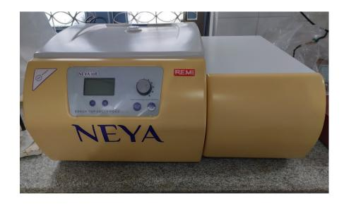
A centrifuge is a piece of equipment that puts an object in rotation around a fixed axis (spins it in a circle), applying a force perpendicular to the axis of spin (outward) that can be very strong. The centrifuge works using the sedimentation principle.
