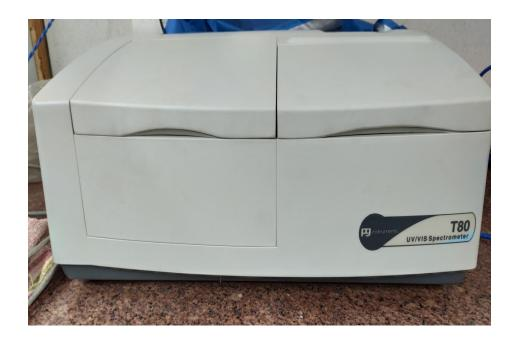
Ultraviolet-visible spectroscopy or ultraviolet-visible spectrophotometry (UV-Vis or UV/Vis) refers to absorption spectroscopy or reflectance spectroscopy in part of the ultraviolet and the full, adjacent visible spectral regions.
