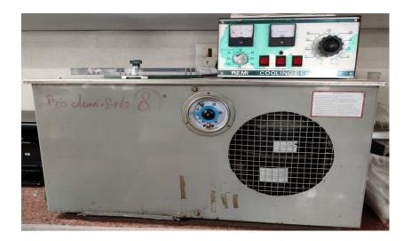
A centrifuge is a device for separating particles from a solution according to their size, shape, density viscosity of the medium and rotor speed. Refrigerated laboratory centrifuges temperature ranges as wide as -20°C - 40°C, making them perfect for DNA, RNA, PCR or antibody analysis.
