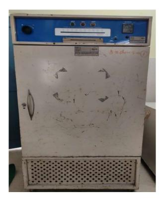
BOD Incubator (Bio-Oxygen Demand) are used to maintain temperature for test tissue culture growth, storage of bacterial cultures and incubation where high degree of constant temperature accuracy is required
