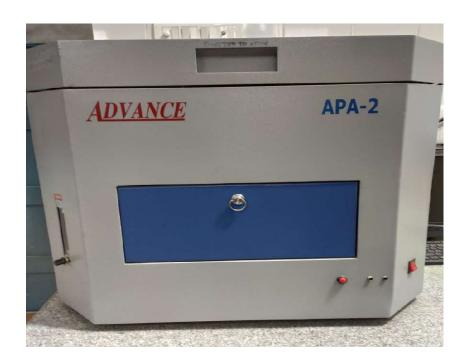
Proximate Analyzer is used to determine the moisture, ash, volatile matter and fixed carbon in coal and coke.
