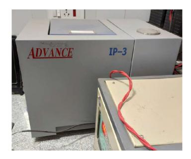
A bomb calorimeter is a type of constant-volume calorimeter used in measuring the heat of combustion of a particular reaction.
