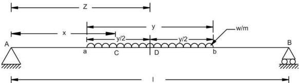
Figure 7.16: Beam loaded with UDL shorter in length than span
