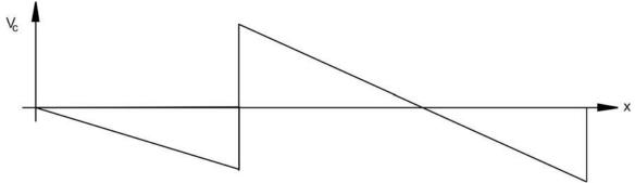
Figure 7.6: Influence line for shear at section C
