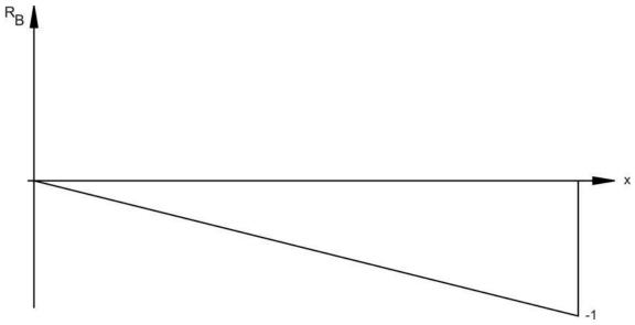
Figure 7.12: Influence line for support reaction at B
