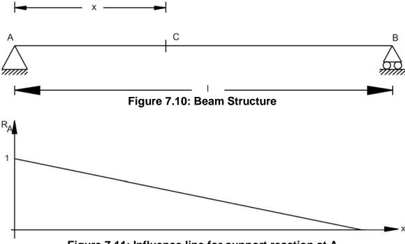
Figure 7.11: Influence line for support reaction at A
