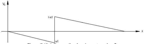
Figure 7.13: Influence line for shear at section C
