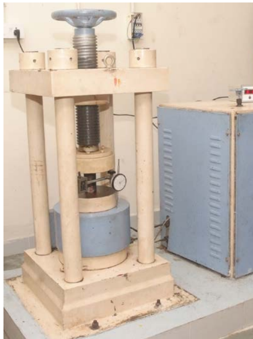
Figure 2.6: UCS test under progress with 200t capacity compression testing machine
