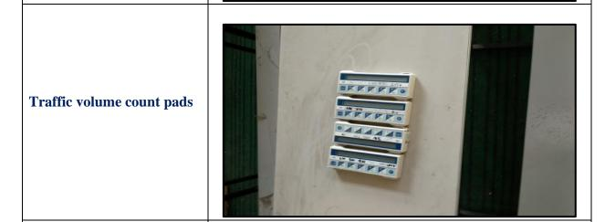
Automatic Pneumatic loop based traffic counts
