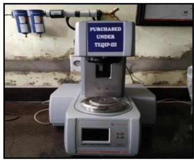
Asphalt Mixture Performance Tester (AMPT)
