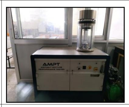
Universal Testing Machine (Servo pneumatic)
