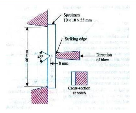
of various materials or toughness of the same material under different condition. This test can also be used to assess the ductile brittle transition temperature of the material occurring due to lowering of temperature.
