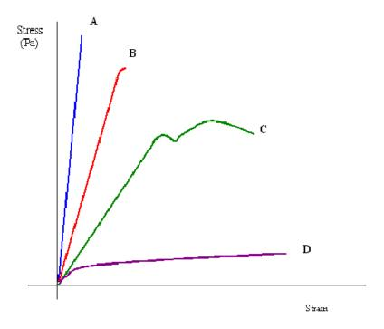
Curve **A** shows a **brittle** material. This material is also strong because there is little strain for a high stress. The fracture of a brittle material is sudden and catastrophic, with little or no plastic deformation. Brittle materials crack under tension and the stress increases around the cracks. Cracks propagate less under compression.
