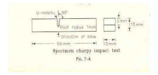
test. The range, within which the pendulum is swinging, is partially protected by the guard. A latch is provided which keeps the pendulum is elevated position.
