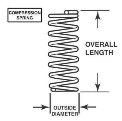
Several types of spring are available for different application. Springs may classified as helical springs, leaf springs and flat spring depending upon their shape. They are fabricated of high shear strength materials such as high carbon alloy steels spring form elements of not only mechanical system but also structural system. In several cases it is essential to idealise complex structural systems by suitable spring.
