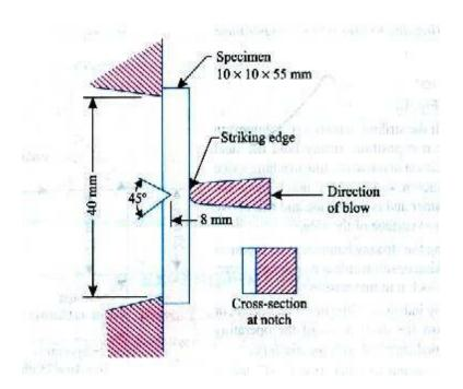
In Izod test, the specimen is placed as cantilever beam. The specimens have V-shaped notch of 45°. U-shaped notch is also common. The notch is located on tension side of Specimen during impact loading. Depth of notch is generally taken as ¬ to ¬ where t is thickness of the specimen.
