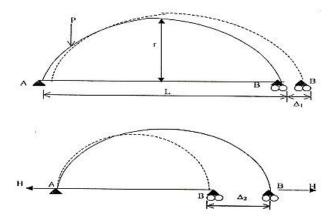
**Theory:** - The two hinged arch is a statically indeterminate structure of the first degree. The horizontal thrust is the redundant reaction and is obtained y the use of strain energy methods. Two hinged arch is made determinate by treating it as a simply supported curved beam and horizontal thrust as a redundant reaction. The arch spreads
