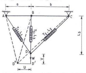
The horizontal (U) and the vertical (V) displacements of the point D is calculated as follows
