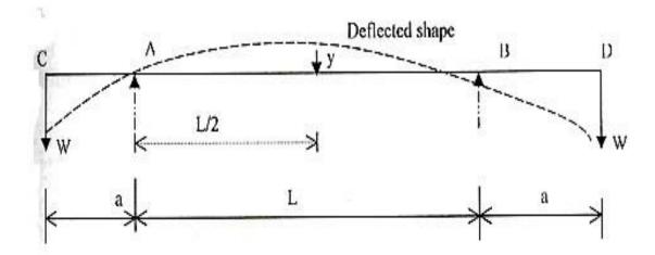
**Theory:** - For the beam with two equal overhangs and subjected to two concentrated loads W each at free ends, maximum deflection y at the centre is given bycentral upward deflection.Central upward deflection,  $y = W.a.L^2 / 8EI$  Where,
