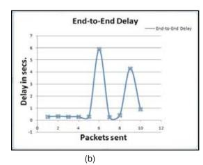
Fig. 6: (a). Shows End-to-End Delay Without Wormhole Attack (b). Shows End-to-End Delay Due to Wormhole Attack
